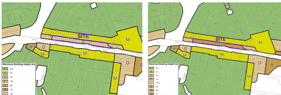
Figure 1. Existing and Proposed Height of Buildings
