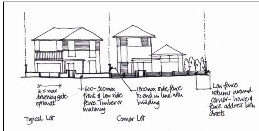
Figure 14 Fence principles in elevation
