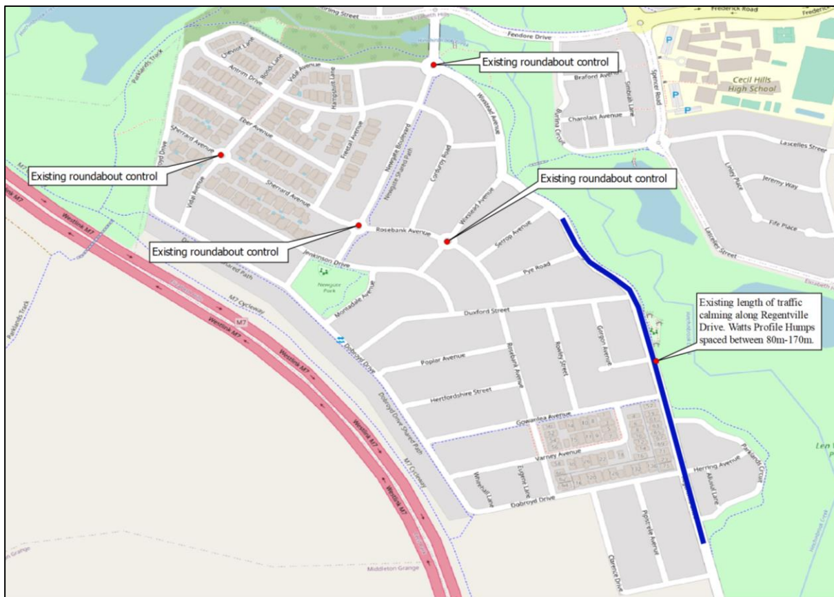
Figure 2.1: Current Traffic Management Facilities
