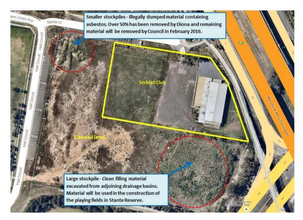
The large stockpile was formed from material that was excavated during construction of the adjacent water detention basin and water quality control basins and is considered to be Virgin Excavated Natural Material (VENM). This material has been stockpiled for use in the upgrading of the reserve.
