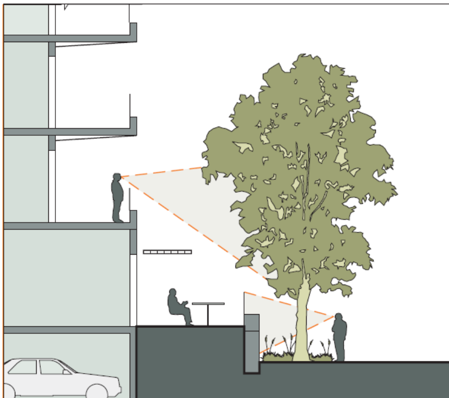
Figure 33: Screening and lower level balconies
