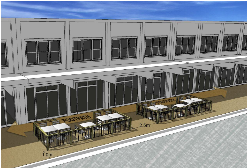
Figure 23 Placement of outdoor seating areas cannot interfere with pedestrian road access
