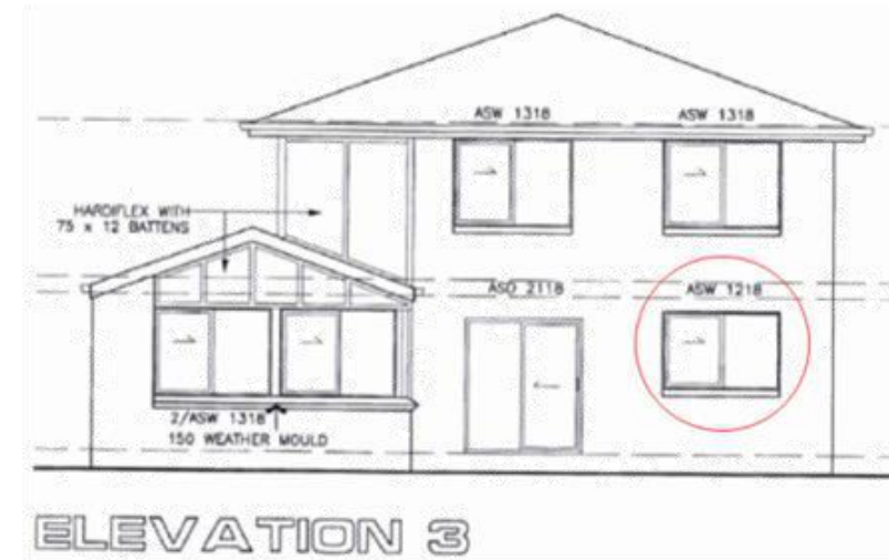
ELEVATION EAST IN ORIGINAL DA-654/00 SHOWING OLD WINDOW ASW1218. SEE SHEET C4.2
