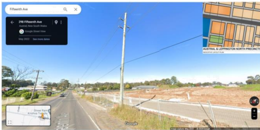
33,000 volt / 33 kilovolt (kV) overhead power lines at Fifteenth Avenue, Austral Source: Google Maps Street View. Inset Austral & Leppington North Precincts Indicative Layout Plan.
