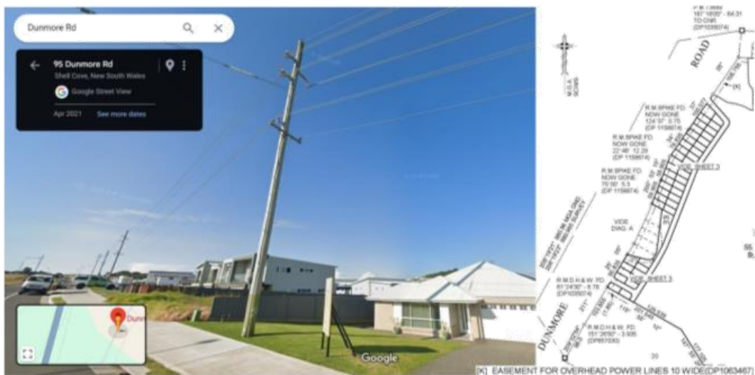
Easement for 11,000 volt / 11 kilovolt (kV) and 33,000 volt / 33 kV overhead power lines at Dunmore Road, Shell Cove. Source: Google Maps Street View. Extract of Deposited Plan DP 1113813.
