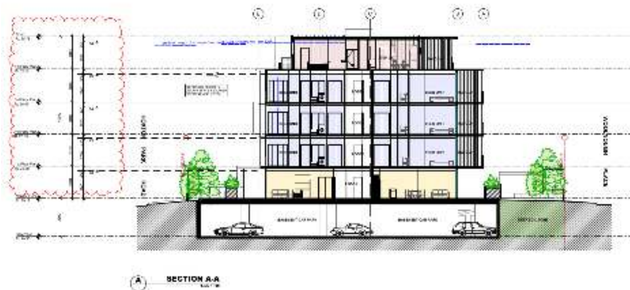
Figure 8: Section plan showing building elements which exceed the 15m height control limit.
