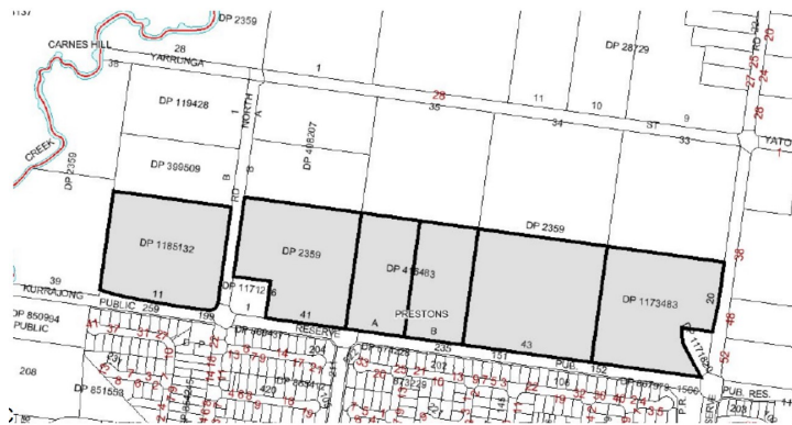
Figure 7: Speed humps are to be provided within the service road to be located on the highlighted lots at 100m intervals.
