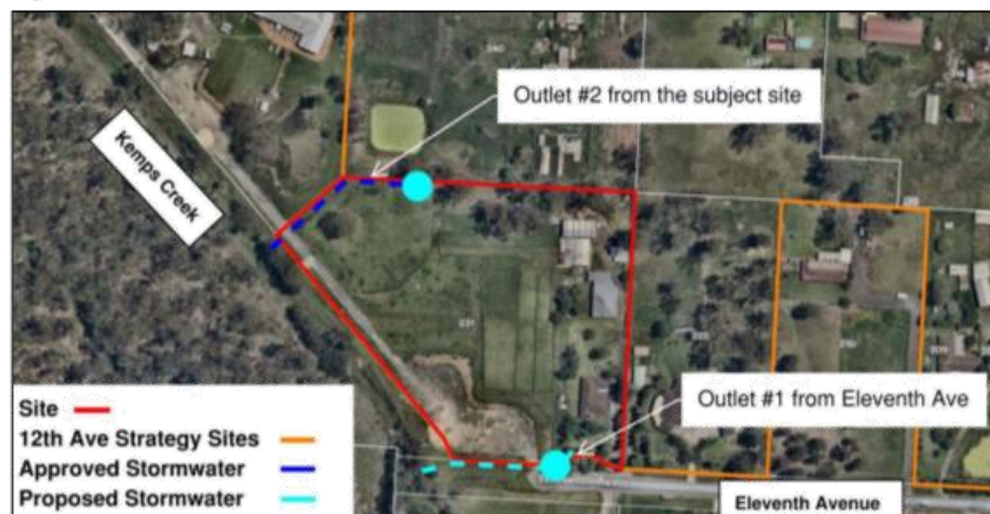
Figure 1.3 Location of Outlets 1 and 2
